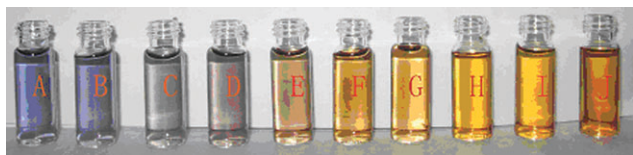
Fig. 4 Different solutions of zincon and copper ions ( 5.0 \times 10^{-5} and 2.2 \times 10^{-5} mol L -1 , respectively) in water in the presence of different concentrations of CN - . From left to right ( \times 10^{-5} mol L -1 ): 0, 1.0, 2.0, 3.0, 4.0, 5.0, 6.0, 7.0, 8.0 and 9.0.
